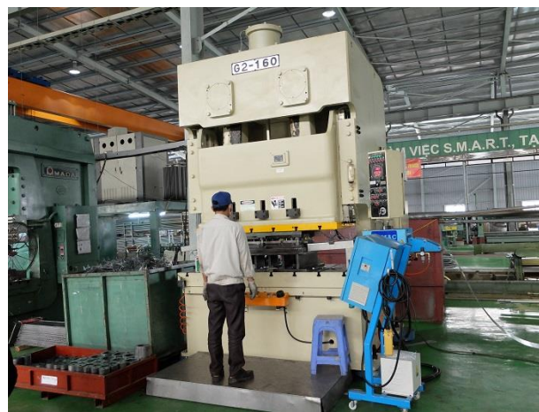
A recently installed press. Its uses include die cutting electromagnetic materials
